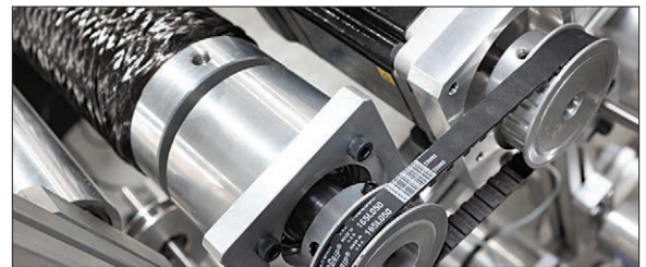
Creel Motor Torque - driven systems with DC servo motors
