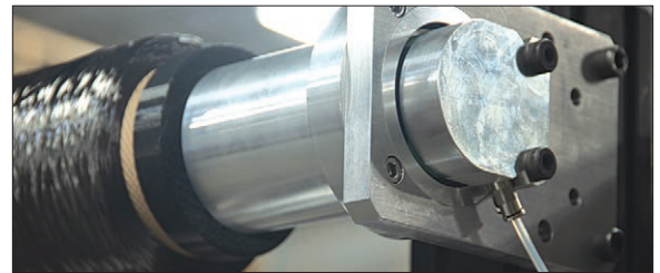
Creel Brake Torque - pneumatically controlled brakes
